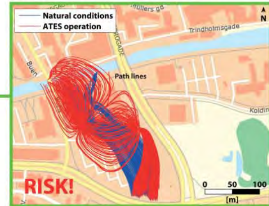
Figure 5: Steady-state particle paths for the existing GW contamination given that water is pumped from the hot storage at the maximum monthly average abstraction rate (12.5 m 3 /h). The contamination reaches the pumping well and is injected back into the aquifer at the cold storage well. Contamination discharges to Kolding Å and to the pumping well at the hot storage, respectively. ATES operation causes significant dispersion of the contamination. Implementation of active remediation in the ATES system should be considered.
